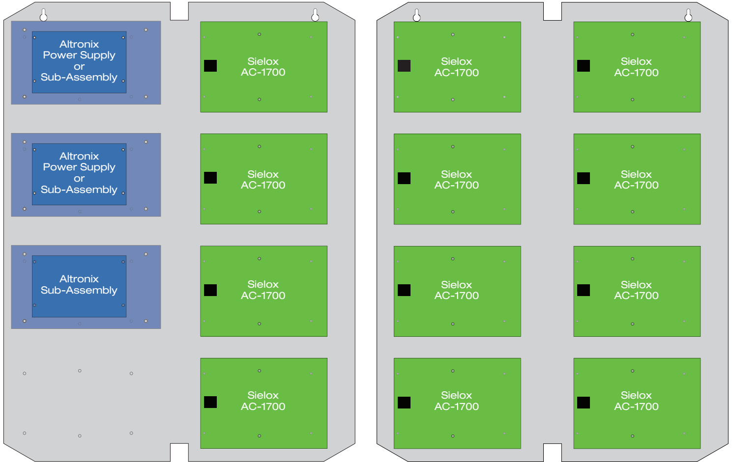
Trove2SL2 Interior Backplane - Optional Mounting Configurations
